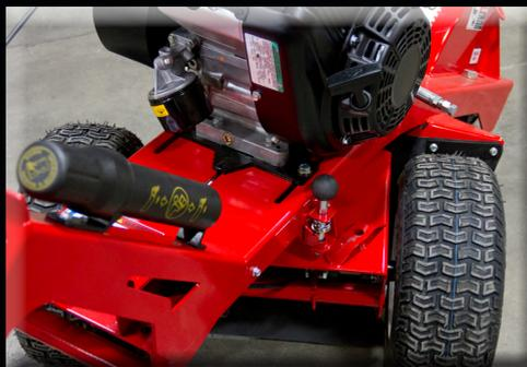
The innovative pivot over center swivel head design allows the grinding wheel to sweep easily across the stump.
